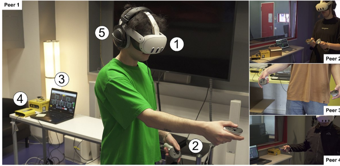
Fig. 6. The equipment used by participants: 1) Meta Quest 3, 2) Tracked controllers; 3) Elk Studio Live; 4) Elk LIVE Bridge; 5) Headphones.
