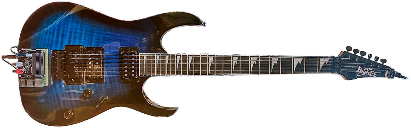
Fig. 5. The developed SMI prototype, with the embedded system and IMU sensor.
