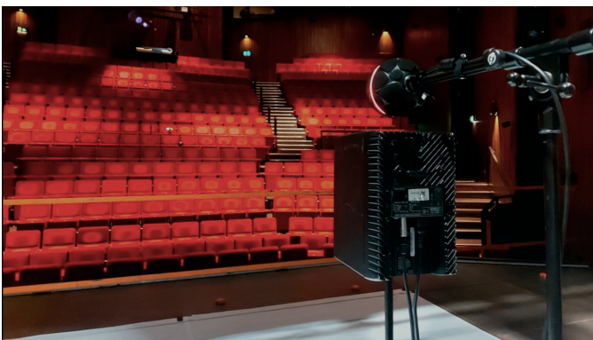
Fig. 3. Loudspeaker and Ambisonics microphone setup during the acoustic capture at the Abbey Theatre.
