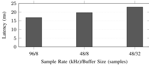
Fig. 20. MM2ME latency measurement results of the TASP over WAN between Stockholm and Oslo
