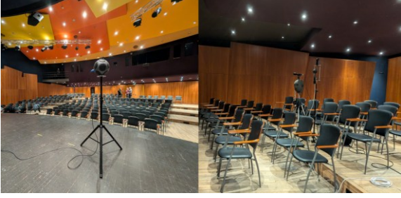
Fig. 3. Example diagram of sound source and receiver setup in Vatroslav Lisinski small Hall.
