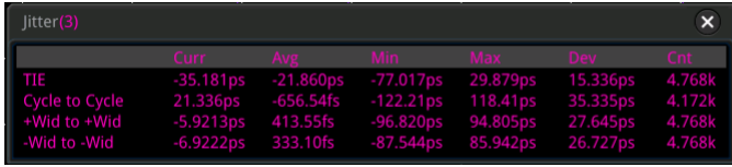
Fig. 16. Jitter table of 49.152 MHz from the oscilloscope
