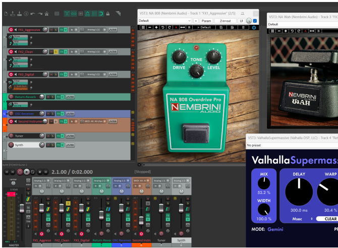
Fig. 3: Screen capture of the DAW, showing a part of the utilized virtual audio effects. Each plugin was selected from cost-free offerings from different developers (e.g., Valhalla DSP, Nembrini Audio). The main three effect scenes were arranged in three tracks. Additional tracks were used for mixing and hosting OSC receivers.
