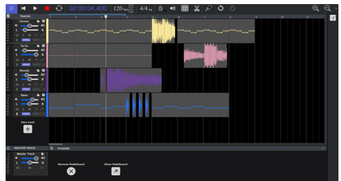
Figure 3: Tracks in WAM-Studio. Regions can be audio or MIDI and can overlap, be moved, deleted, split, merged, etc.
