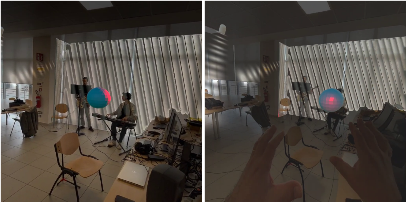
Fig. 5: Two captures from the XR headset during a session with two musicians. The stripes in the background, the light flares on the left, and the shape of the metaball in the center of the visual field are all virtual elements that were influenced by passive BCI signals. The computer monitor in front of the guitar player was used to display the BCI-console interface for active sound control.
