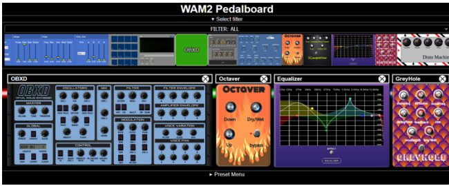
Figure 6: The WAM-bank plugin that manages chains of plugins (virtual instruments and audio effects) associated with each track.
