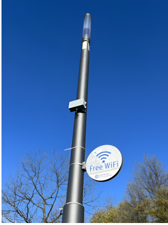
Fig. 3: Acoustic sensor (grey box) mounted on a lamppost in the Open Innovation Lab area at Gelsenkirchen. Photo: comNET GmbH
